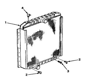
a. Wrap threads with two turns of teflon
