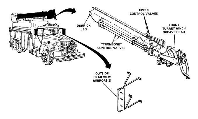
Upper control valves are attached to the front turret winch sheave head. Derrick leg elevation, rotation, and extension are controlled from the main basket with the hydraulically powered upper control valves.
