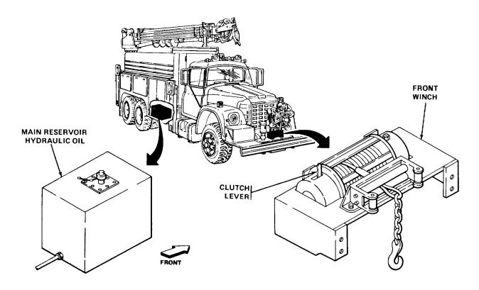
The front winch is hydraulically powered and driven by a hydraulic motor. Winch engagement of the hydraulic motor is controlled by a clutch lever on the winch housing. Takeup and payout of winch cable is controlled from the driver's position.
