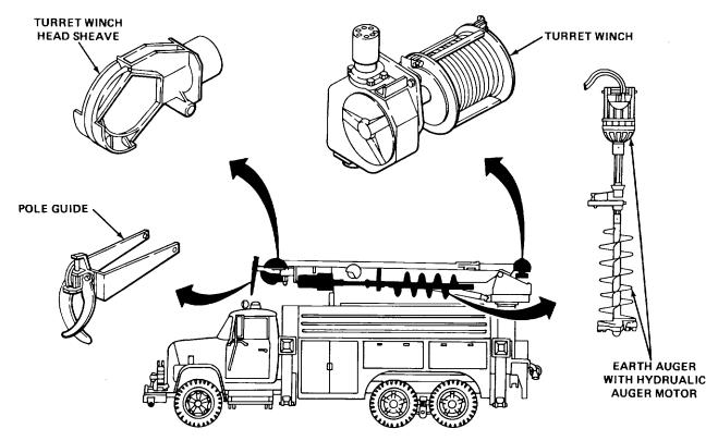
The earth auger digs the telephone pole holes. It is hydraulically driven and is controlled from the operator's station. The earth auger with hydraulic motor is attached to the left side of the derrick boom and is self-storing. The earth auger is capable of forward and reverse drilling speeds.
