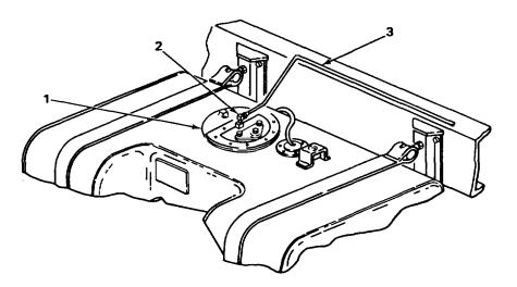
Step 7. Test fuel supply lines (3), (4), and (5) for blockage.
