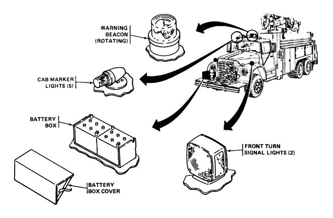
The battery box and cover are formed from heavy gage steel and house two 12-volt batteries for vehicle starting power.
