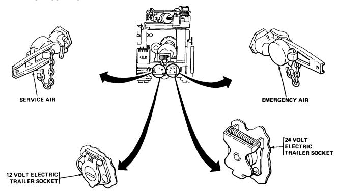
The 12-volt electric trailer socket provides power to operate trailers having a 12-volt electrical brake system and is controlled by a switch on the cab instrument panel.
