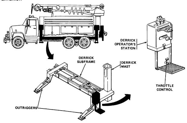
The derrick subframe is steel fabricated and welded into one unit. Subframe includes derrick mast, outriggers, and derrick operator's control console. The subframe mounts on and is bolted to the M876 Truck frame. The subframe derrick mast supports the derrick and distributes loads to the M876 Truck frame.
