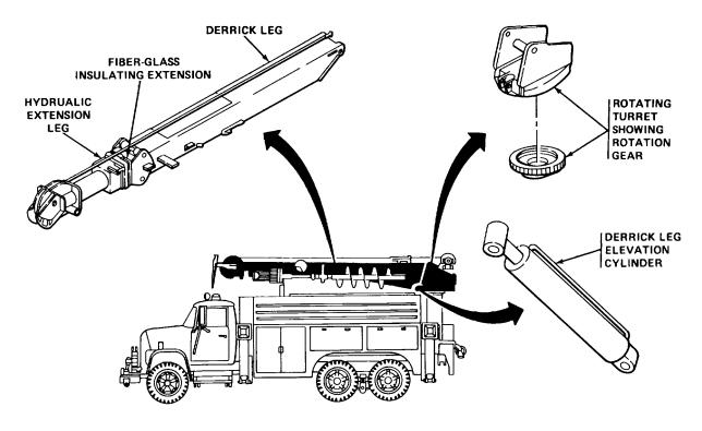
The rotating turret mounts on top of the derrick mast, and the rotation gear is driven by a hydraulically powered motor. The turret rotates to 360 degrees right and left direction only, non-continuous, and is controlled from the operator's station.
