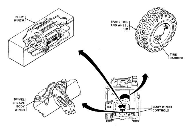
The body winch is mounted and bolted to the derrick subframe at the front section of the maintenance body. The hydraulically powered winch is controlled from the right rear side of the M876 Truck by individual winch controls.
