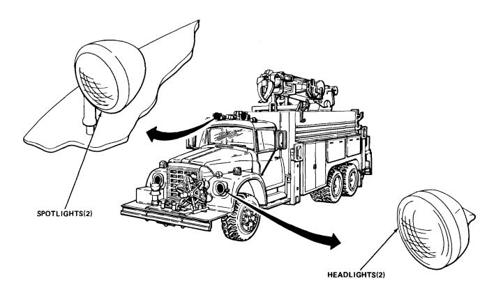
The two (2) headlights provide illumination for night driving and are controlled by a switch on the cab instrument panel and a floor foot control.
