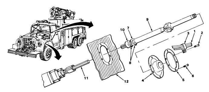
Two nuts (8) and U-bolt (7) Using 9/16-inch socket and handle, unscrew and take off. 7. Clamp (13) 8. Drive shaft (9) Boot (10) and Take apart. clamp (13) **INSTALLATION**
