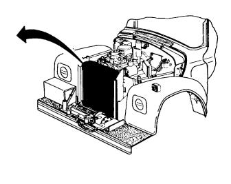
a. Using 1 1/16-inch and 1 1/4-inch wrenches, unscrew and take off.
