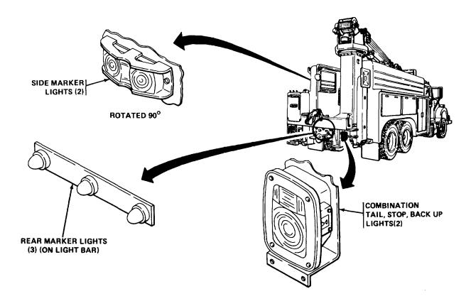
The two (2) rear side marker lights provide illumination Indicating vehicle body clearance width during night driving, as required by FMVSS, and are controlled by the headlight switch on cab dash panel.
