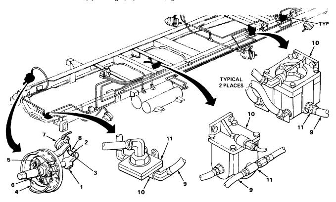
Step 6. Inspect wheel bearings, drums, and wheel sensors.
